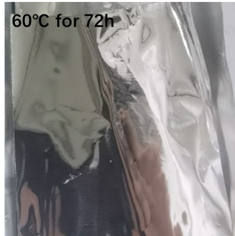
Supplementary Figure S6. Morphology of Al-PET stored in EC/DEC electrolyte at 25 °C and 60 °C for 72 h.
