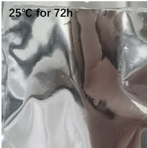
Supplementary Figure S6. Morphology of Al-PET stored in EC/DEC electrolyte at 25 °C and 60 °C for 72 h.
