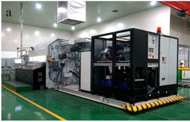
Supplementary Figure S1 (a) The vacuum-metallizing machine used and (b) the schematic of Al deposition for the roll-to-roll preparation of Al-PET.
