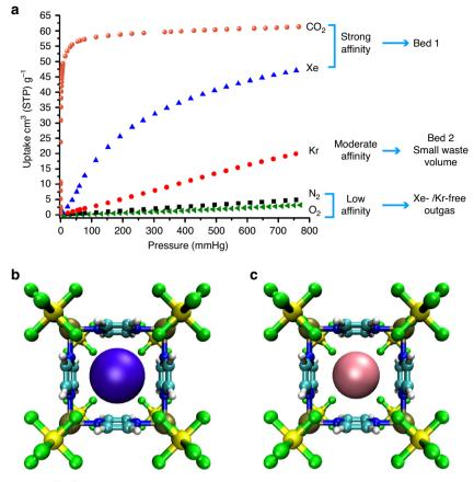
**Fig. 4 Gas adsorption properties and binding sites. a** Single-component CO<sub>2</sub>, Xe, Kr, N<sub>2</sub>, and O<sub>2</sub> adsorption isotherms at 298 K for SIFSIX-3-Cu. Molecular illustration of the most favorable binding site for **b** Xe and **c** Kr in SIFSIX-3-Cu (top view) as determined from simulated annealing calculations. Atom colors: C = cyan, H = white, N = blue, F = green, Si = yellow, Cu = gold, Xe = violet, Kr = pink.
