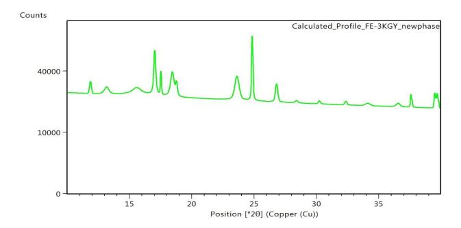
**Supplementary Figure 6.** Calculated profile for the new phase appears after irradiation of SIFISIX-3-Fe with 3 kGy.
