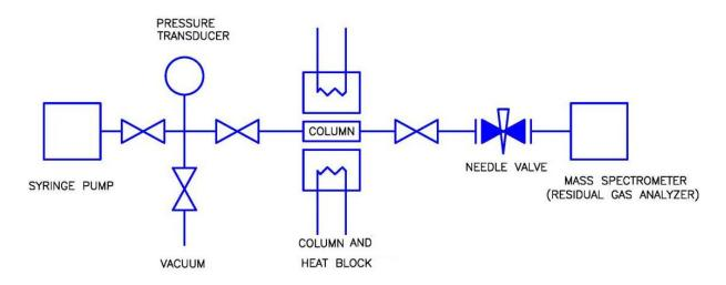
**Supplementary Scheme 1.** Schematic representation of the single column breakthrough experiment set-up combined with the mass spectrophotometer.
