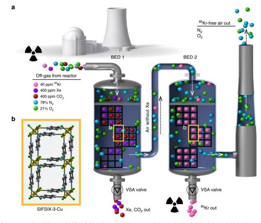
**Fig. 1 Schematic representation of the two-bed breakthrough setup. a** Illustration of the two-bed technique for removal of radioactive Kr from nuclear reprocessing plants using SIFSIX-3-Cu. **b** Each two squares in the bed 1 and bed 2 represent two channels of SIFSIX-3-Cu structure. Atom colors: C = gray, H = white, N = light blue, F = green, Si = light brown, Cu = orange, O = red, Xe = violet, Kr = pink.
