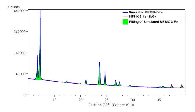
**Supplementary Figure 5.** Rietveld fitting method between SIFSIX-3-Fe crystal structure (blue) and irradiated structure at 1 kGy (red).
