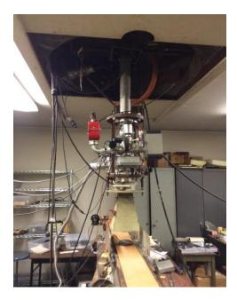
Supplementary Figure 18. Van deGraaff electron accelerator.
