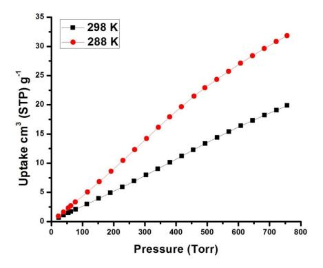
**Supplementary Figure 20.** Single component Kr sorption isotherms for SIFSIX-3-Cu measured at 298 K and 288 K.
