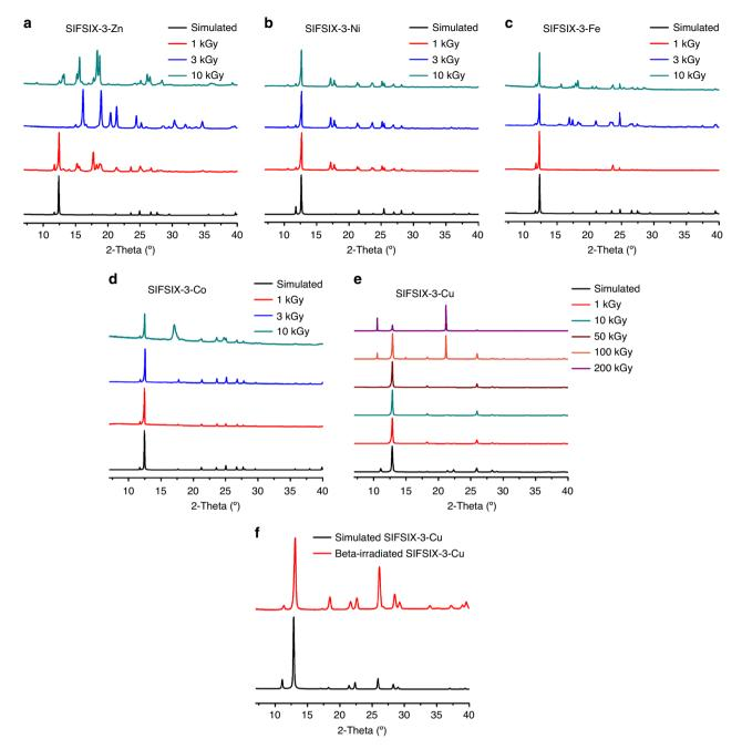
Fig. 3 Powder X-ray diffraction patterns of irradiated and simulated SIFSIX-3-M structures. a gamma-irradiated SIFSIX-3-Zn, b gamma-irradiated SIFSIX-3-Ni, c gamma-irradiated SIFSIX-3-Fe, d gamma-irradiated SIFSIX-3-Co, and e SIFSIX-3-Cu and f activated SIFSIX-3-Cu structure after 50 kGy beta irradiation.
