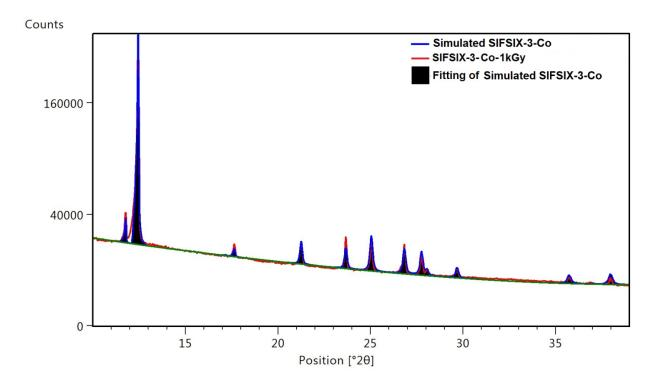
**Supplementary Figure 9.** Rietveld fitting method between SIFSIX-3-Co crystal structure (blue) and irradiated structure at 1 kGy (red). Baseline is shown in green.
