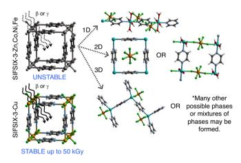
**Fig. 2 Illustration of impact of irradiation on SIFSIX-3-M materials.** The SIFSIX-3-M (M = Zn, Co, Ni, Fe) structures decompose to 1D, 2D or many other possible phases up on radiation exposure. The SIFSIX-3-Cu is stable and maintains its original crystal structure up to 50 kGy dose in beta or gamma radiation. Atom colors: C = gray, H = white, N = light blue, F = green, Si = light brown, Cu = orange, M (Ni, Co, Fe, Zn) = cyan, O = red.
