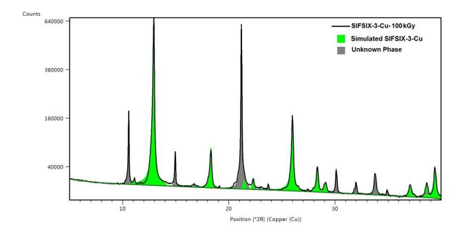
**Supplementary Figure 16.** Pawley fitting method between SIFSIX-3-Cu crystal structure and irradiated one at 100 kGy.
