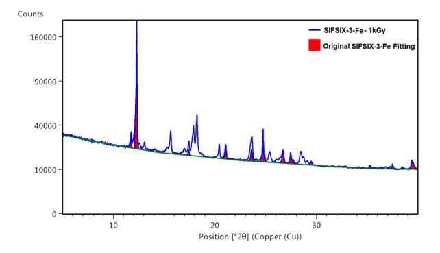
**Supplementary Figure 8.** Pawley fitting method between SIFSIX-3-Fe crystal structure and irradiated one at 10 kGy (green color for the baseline).
