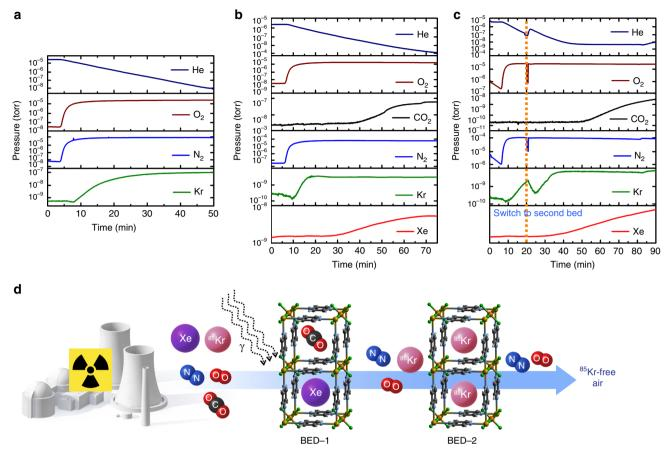
**Fig. 5 Breakthrough curves for SIFSIX-3-Cu. a** Single-bed breakthrough experiment using 1000 ppm Kr balanced with dry air. **b** Single-bed breakthrough experiment using 400 ppm Xe and 40 ppm Kr balanced with dry air. **c** Two-bed breakthrough experiment using 400 ppm Xe and 40 ppm Kr balanced with dry air. **d** schematic demonstration of the concept of the two-bed technique for the <sup>85</sup>Kr removal from the UNF.
