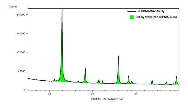
**Supplementary Figure 14.** Pawley fitting method between SIFSIX-3-Cu crystal structure and irradiated one at 10 kGy.
