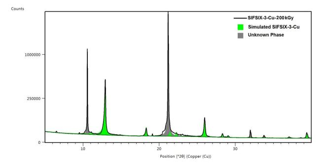
**Supplementary Figure 17.** Pawley fitting method between SIFSIX-3-Cu crystal structure and irradiated one at 200 kGy.
