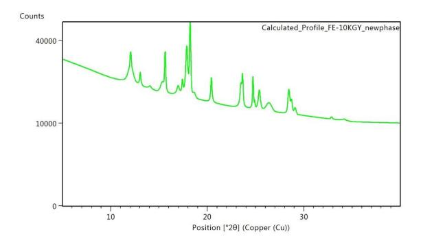
**Supplementary Figure 7.** Calculated profile for the new phase appears after irradiation of SIFISIX-3-Fe with 10 kGy.
