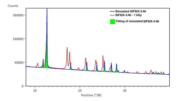
**Supplementary Figure 4.** Pawley fitting method between SIFSIX-3-Ni crystal structure (blue) and irradiated one at 1 kGy (red).
