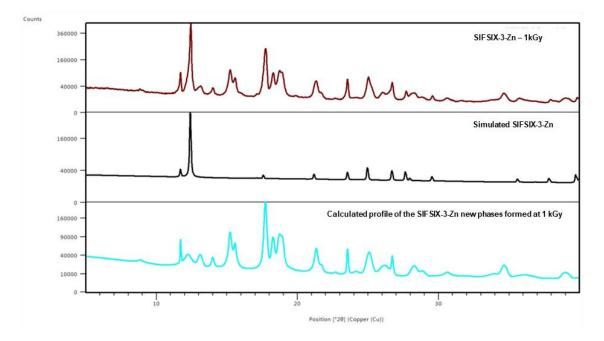
Supplementary Note 2. Powder X-ray diffraction after gamma irradiation
