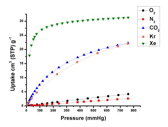
**Supplementary Figure 22.** Single component Xe, CO<sub>2</sub>, Kr, O<sub>2</sub> and N<sub>2</sub> sorption isotherms for SBMOF-1 measured at 298 K demonstrating extremely low Kr/CO<sub>2</sub> selectivity.
