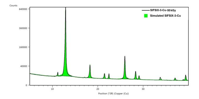
**Supplementary Figure 15.** Pawley fitting method between SIFSIX-3-Cu crystal structure and irradiated one at 50 kGy.
