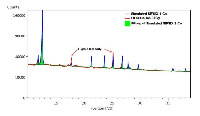
**Supplementary Figure 10.** Rietveld fitting method between SIFSIX-3-Co crystal structure (blue) and irradiated structure at 3 kGy (red).
