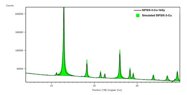
**Supplementary Figure 13.** Pawley fitting method between SIFSIX-3-Cu crystal structure and irradiated one at 1 kGy.
