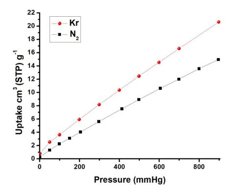
Supplementary Figure 21. Single component Kr and  $N_2$  sorption isotherms for Ni-MOF-74 measured at 298 K demonstrating the low Kr/N<sub>2</sub> selectivity.
