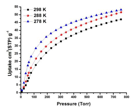
**Supplementary Figure 19.** Single component Xe sorption isotherms for SIFSIX-3-Cu measured at different temperatures.
