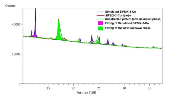
**Supplementary Figure 12.** Pawley fitting method between SIFSIX-3-Co crystal structure (blue) and irradiated structure at 10 kGy (red). To quantitatively analyze the two superimposed XRD patterns we apply both Rietveld and Pawley fitting methods to the SIFSIX-3-Co and the unknown phase, respectively. The Pawley method is used to obtain structure factors by fitting the peak intensities independently.
