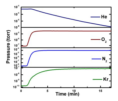
Supplementary Figure 30. Single-bed breakthrough experiment using 1000 ppm Kr balanced with dry air for Ag mordenite demonstrating the low  $Kr/N_2$  selectivity.
