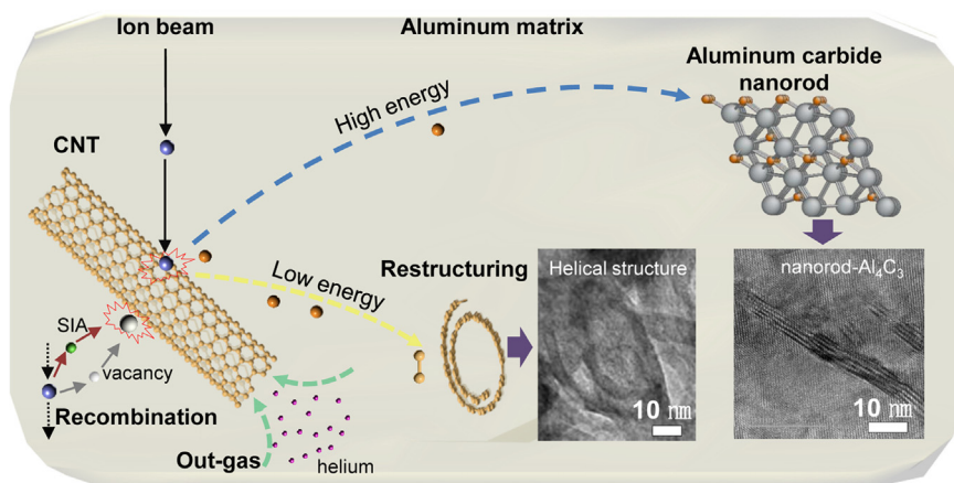
Figure 1 Schematic illustration of shape changes on CNT, recombination, and helium out-gas. Under ion irradiation, the disintegration of CNT and formation of aluminum carbide (blue arrow) from high energy ion and restructuring to helical CNT structure (yellow arrow) from low energy ion are indicated.
