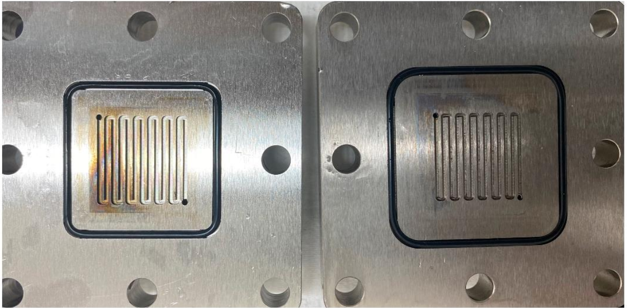
Fig. S5. The flow field of a 5 cm 2 membrane electrode assembly electrolyzer.
