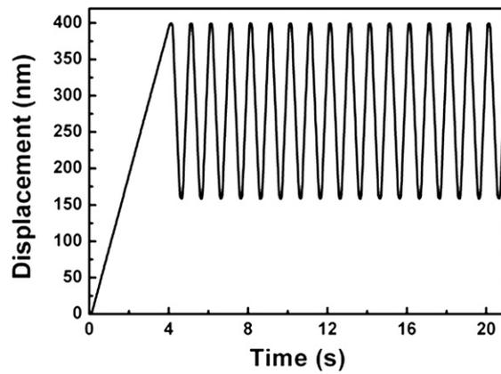
**Fig. S10.** Displacement-controlled cyclic straining testing with a frequency of 1 Hz and the triangular waveform used in all of the fatigue experiments reported in this work for the test geometry shown in Fig. 1A of the main text.
