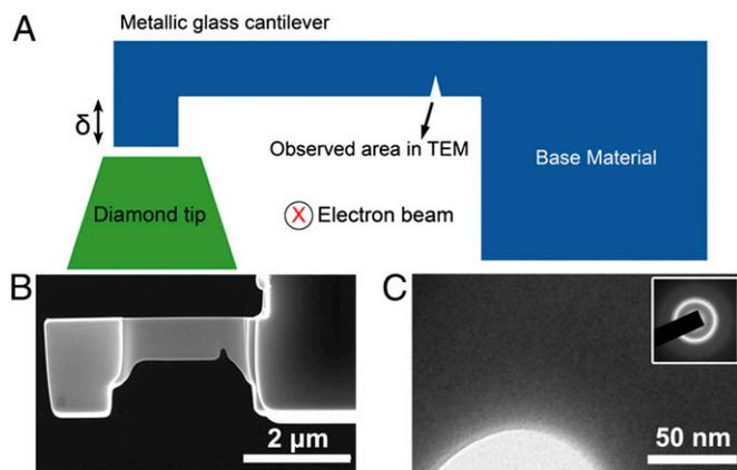
**Fig. 1.** In situ fatigue testing of the metallic glass inside a TEM. (A) Schematic of the experimental setup. Note that the electron beam direction is perpendicular to the plane. (B) SEM image showing a sample fabricated by a FIB. (C) Bright-field TEM image of the notch tip before testing shows that the sample has a fully amorphous structure, as evidenced by the SADP (Inset).
