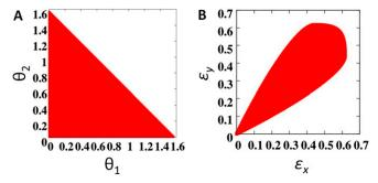
Fig. S2. Allowable hinge angles and strains in the level-2 structure. (A) The allowed angles  $\theta_1$  and  $\theta_2$  for the level-2 structure are shown in red. (B) The strains  $\varepsilon_x$  and  $\varepsilon_y$  that are realizable in the level-2 structure.
