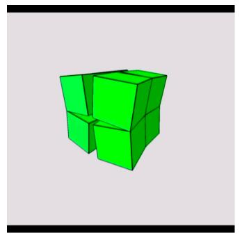
Movie S4. Stretching of the level-1 three-dimensional cubic structure [using the rigid unit, finite stiffness corner hinge model in Bullet Physics (1)].
