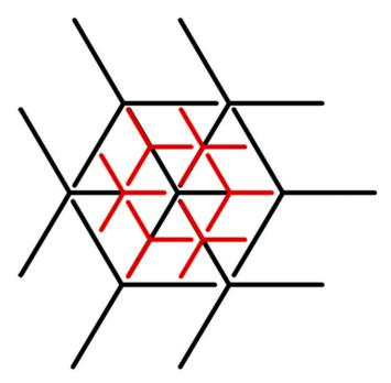
Fig. S6. Triangular (kagome) pattern. Black lines represent a level - kagome pattern breaking the material into six rotating triangular units. Red lines represent a level-2 kagome pattern. Similar to the square units in which different motifs may be obtained by a 90° rotation of the cut pattern, a different motif of the kagome pattern can be obtained by 60° rotation of the original cut pattern.
