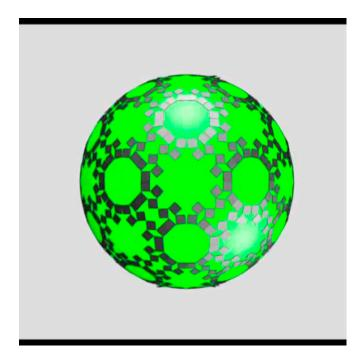
Movie 56. Conformal draping of a sphere by a two-dimensional fractal cut material with level-3 fractal cut structure [using the rigid unit, finite stiffness hinge model in Bullet Physics (1)].
