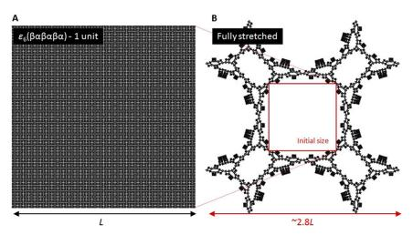
Fig. S4. (A) The level-6 (βαβαβα) structure at the maximum biaxial strain obtained using the finite element method. (B) The initial (unstretched) sample size.
