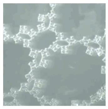
**Movie S1.** Releasing the stretched PDMS sheet. The stretched level 4 ( $\beta\alpha\beta\alpha$ ) being released from the glass substrate by the addition of ethanol.
