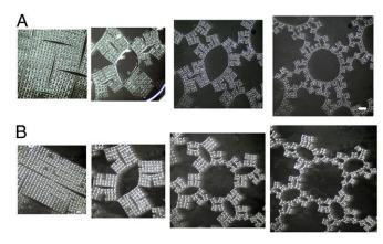
Fig. 5. Microscopic experimental realization. PDMS sheets differentiated with patterned cuts. The smallest feature size (hinge width) is 40 µm. (A) One unit of the homogeneous  $\varepsilon_4(\alpha\alpha\alpha\alpha)$ . (B) One unit of the  $\varepsilon_4(\beta\alpha\beta\alpha)$ . The correspondence between finite element simulation, macroscopic experiment, and microscopic experiment is excellent (cf. Figs. 2, 4, and 5). (The white line in the expanded structure image is 200 µm.)
