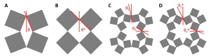
Fig. S1. Ideal geometry with rigid units and free hinges. Four rotating units in the level-1 structure at a (A) small strain and (B) at the maximum lateral strain. Sixteen rotating units in a level-2 structure corresponding to a (C) small biaxial strain and (D) at the maximum biaxial strain.
