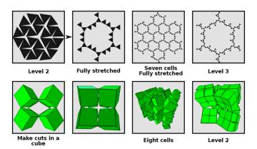
Fig. S7. Nonsquare units. The first row shows level-2 and level-3 expansions of (two-dimensional) kagome structures. The second row demonstrates level-1 and level-2 expansion of three-dimensional cubic units with corner hinges. These calculations were performed using the open source Bullet Physics software (1) (with an arbitrary rotational spring constant) (see also Movies S2–S5).
