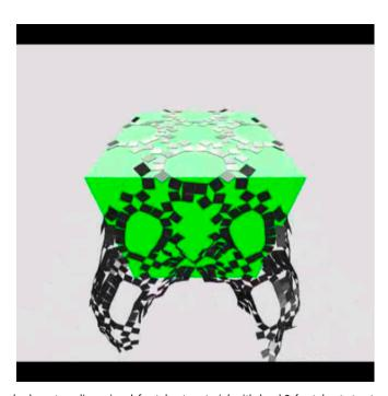
Movie 57. Conformal draping of a cube by a two-dimensional fractal cut material with level-3 fractal cut structure [using the rigid unit, finite stiffness hinge model in Bullet Physics (1)].
