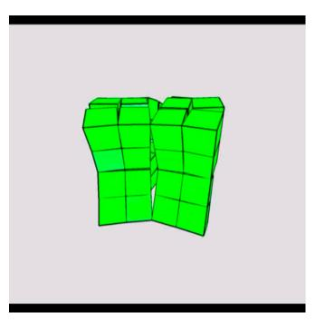
Movie S5. Stretching of the level-2 three-dimensional cubic structure [using the rigid unit, finite stiffness corner hinge model in Bullet Physics (1)].
