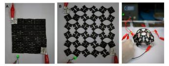
Fig. S8. Stretchable electrode on a silicone rubber substrate with a level-3 fractal cut pattern. (A) A green LED connected to a battery through a series circuit including the fractal cut electrode before stretching. (B) The LED light continues to be powered thorough the stretchable electrodes as the substrate is stretched to ~43% lateral strain and (C) wrapped over the baseball (a nonzero Gauss curvature shape).
