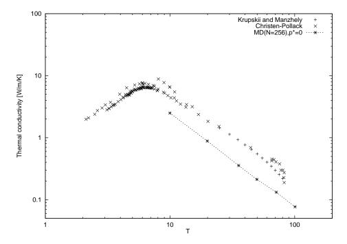
FIG. 1. Thermal conductivity of solid Argon as a function of temperature at free standing condition.
