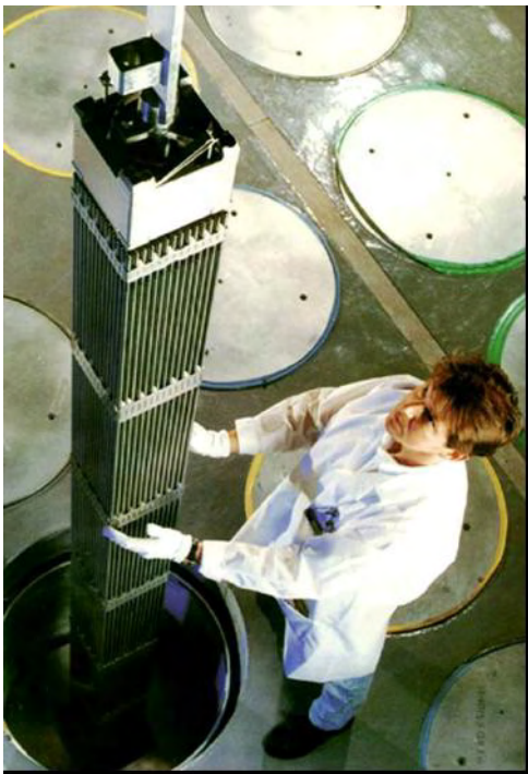
Fig. 2.2. Fabricated fuel rods are bundled into a fuel assembly, which becomes the basic unit for handling fuel. Shown here is a nuclear fuel assembly for a light water reactor.
