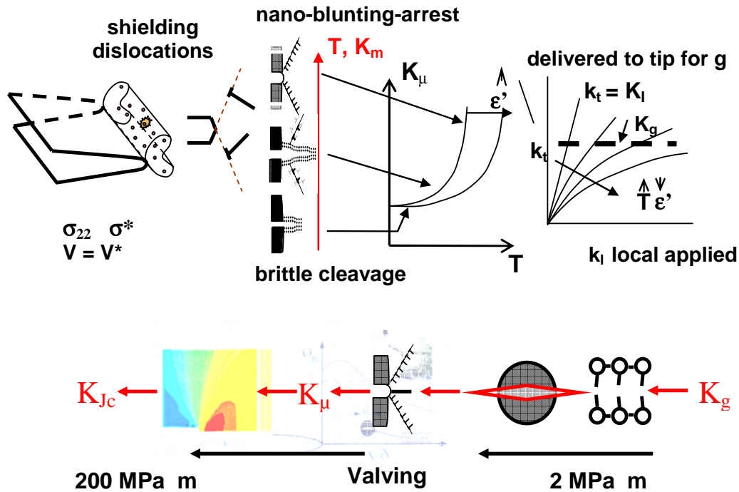
Figure 2: Schematic illustration of the mechanisms controlling brittle failure and the microstructural processes by which local cleavage fracture toughness is amplified. (Odette, G. R., T. Yamamoto, H. J. Rathbun, M. Y. He, M. L. Hribernik, and J. W. Rensman. 2003. "Cleavage Fracture and Irradiation Embrittlement of Fusion Reactor Alloys: Mechanisms, Multiscale Models, Toughness Measurements and Implications to Structural Integrity Assessment," Journal of Nuclear Materials 323, 313.)
