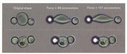
OPTICAL TWEEZERS stretch a healthy red blood cell (top row), increasing the applied force slowly, by a matter of piconewtons. A cell in a late stage of malarial infection is stretched in a similar fashion (bottom row). The experiment illustrates how the infected cell becomes rigid, which prevents it from traveling easily through blood capillaries and helps cause the symptoms of malaria.
