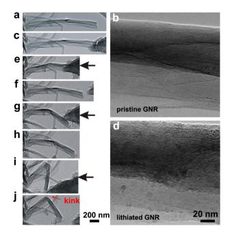
Fig. 5 – Mechanical robustness of a lithiated GNR. (a and b) Pristine GNR. (c and d) Lithiated GNR. (e and j) Morphology change of the lithiated GNR in the three compression-release cycles. Although the lithiated  ${\rm Li}_2{\rm O}/{\rm GNR}$  did not return to the straight morphology after mechanical manipulation, neither did it fracture. The red arrow marks the permanent kink formed during the mechanical manipulation.
