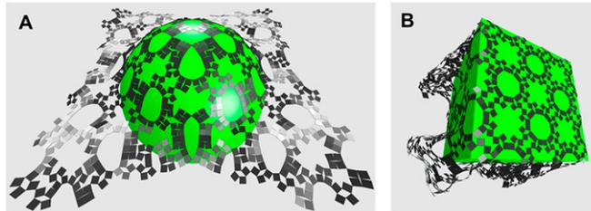
**Fig. 59.** Conformal wrapping of nonzero Gauss curvature object. A level-3 square unit fractal cut structure wrapped around (A) a sphere and (B) a cube. The calculations were performed using the rigid unit and angular hinge model via the open source Bullet Physics software (1) (with an arbitrary rotational spring constant). See [Movies S6](#) and [S7](#) for the draping dynamics.
