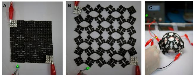
**Fig. 58.** Stretchable electrode on a silicone rubber substrate with a level-3 fractal cut pattern. (A) A green LED connected to a battery through a series circuit including the fractal cut electrode before stretching. (B) The LED light continues to be powered through the stretchable electrodes as the substrate is stretched to  $\sim 43\%$  lateral strain and (C) wrapped over the baseball (a nonzero Gauss curvature shape).
