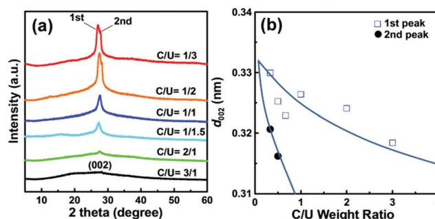
Fig. 4 (a) Typical XRD patterns of all CND samples and (b) corresponding interlayer spacing distances as a function of C/U weight ratio.
