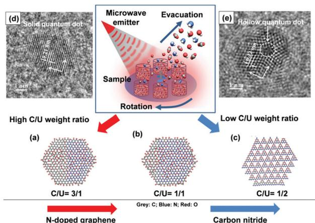
Fig. 5 Schematic diagram of 2D atomic structures created during SPMA process with C/U weight ratios of (a) 3/1, (b) 1/1, and (c) 1/2, simulated by the MD software. HR-TEM micrographs for the CNDs prepared with C/U ratios of (e) 3/1 and (f) 1/2.
