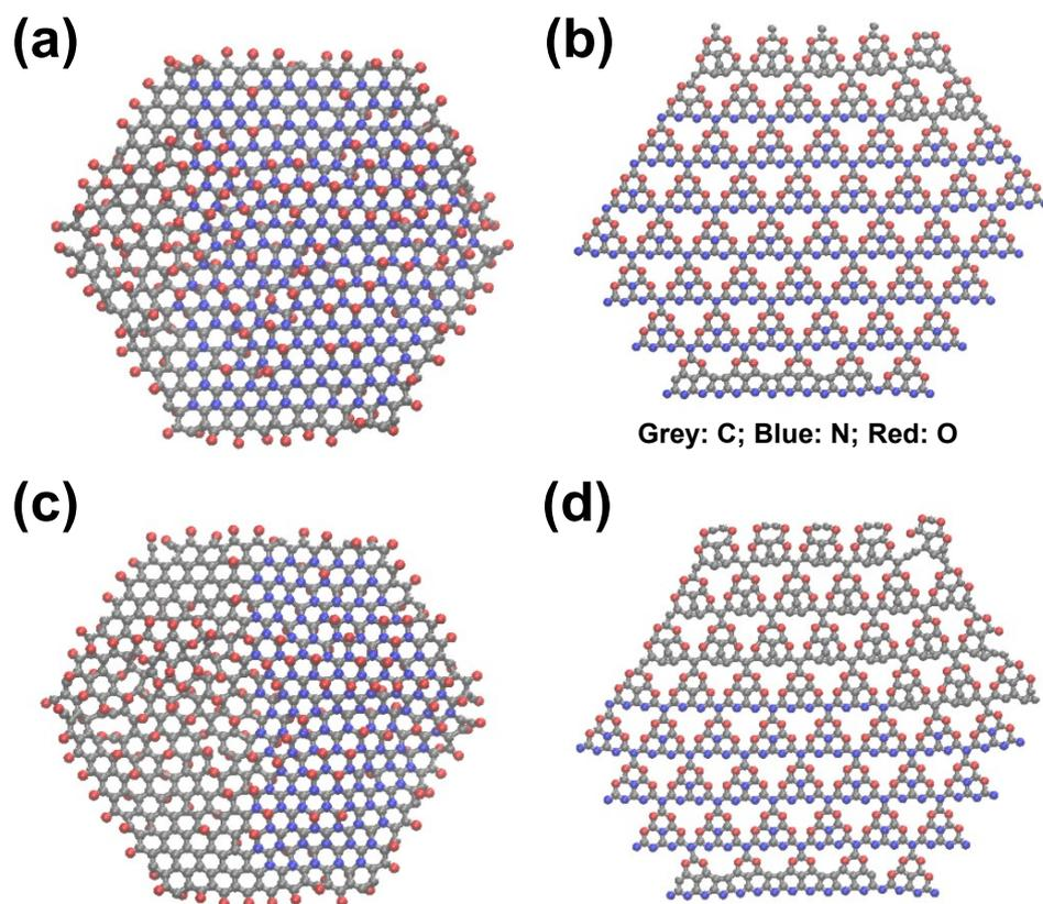
Figure S5. Proposed atomic configurations of 740-atom models with different N/C ratios: heavily N-doped graphene with O adsorption: (a)  $N/C = 24/49$  and (c)  $N/C = 15/53$  and heavily O-doped  $g\text{-C}_3\text{N}_4$ : (b)  $N/C = 24/49$  and (d)  $N/C = 15/53$ .
