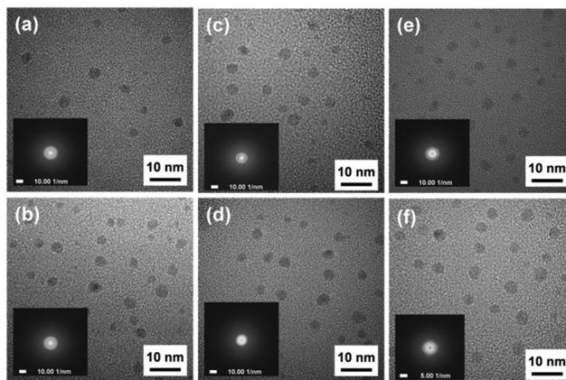
Fig. 1 HR-TEM micrographs of N-doped CND samples prepared using the SPMA method with C/U weight ratios of (a) 3/1, (b) 2/1, (c) 1/1, (d) 1/1.5, (e) 1/2, and (f) 1/3. Inset show the corresponding selected-area diffraction.
