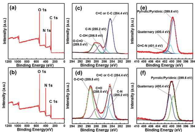
Fig. 2 XPS survey scan, C 1s, and N 1s spectra of N-doped CND samples for C/U ratios of (a, c and e) 3/1 and (b, d and f) 1/3.
