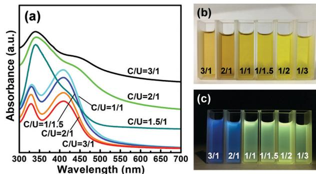
Fig. 6 (a) UV-vis absorption spectra of all CND samples in distilled water and photographs of each CND suspension under (b) visible light and (c) UV illumination at 360 nm.
