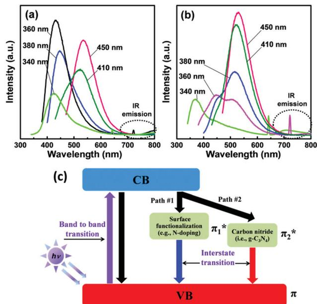
Fig. 7 PL emission spectra of various CND suspensions prepared using SPMA route with C/U ratios of (a) 3/1 and (b) 1/3, excited at different wavelengths. (c) Band-gap structure describing the ( $\pi^*$ - $\pi$ ) transition of CND samples, where CB and VB represent conduction and valence bands, respectively.
