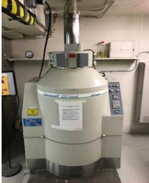
**Supplementary Figure 1.** Gammacell 220 Excel Irradiator.
