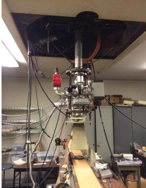
**Supplementary Figure 18.** Van deGraaff electron accelerator.
