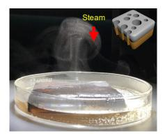
**Supplementary Figure 2.** Photograph of steam generation process from the surface carbonized wood under light illumination.
