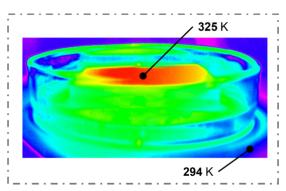
**Figure RR12** (*i.e.*, Figure 1e in the original version). Infrared radiation thermal image from the wood/CoO system under light illumination.
