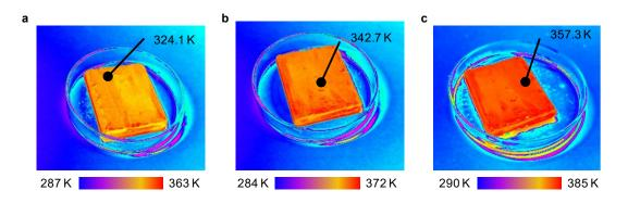
Supplementary Figure 9. Infrared radiation thermal images of the wood/CoO system under light illumination with different solar intensity. **a** 100 mW cm<sup>-2</sup>, **b** 200 mW cm<sup>-2</sup>, **c** 300 mW cm<sup>-2</sup>.
