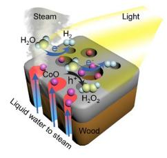
Figure RR8. Schematic of the photocatalytic reaction process of the wood/CoO system.
