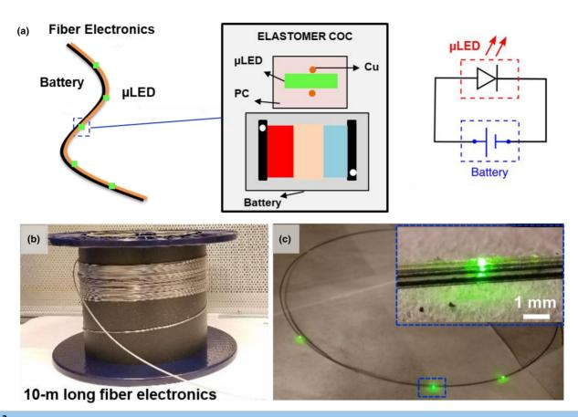
Thermally drawn fiber battery in 1D electronics; Integrated fiber battery through co-drawing of LED and battery modalities; (a) schematic diagram of integrated LED/battery fiber and its corresponding electrical circuit, (b) the 10-meter-long LED/battery fiber, (c) green LEDs powered by fiber battery within the same fiber.
