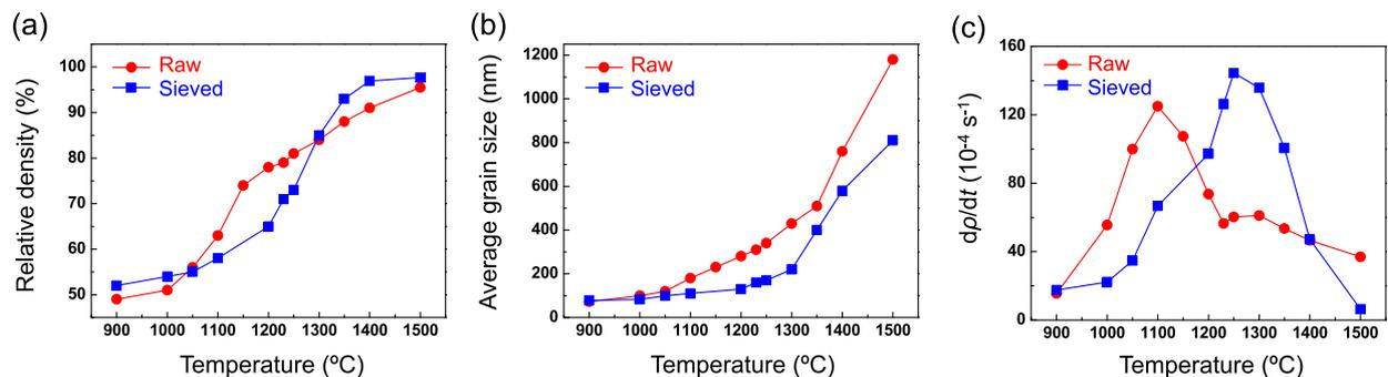
Fig. 3. (a) Relative density  $\rho$ , (b) average grain size  $G_{avg}$ , and (c) sintering rate  $dp/dt$  of samples using raw and sieved powders in constant-heating-rate sintering experiments.
