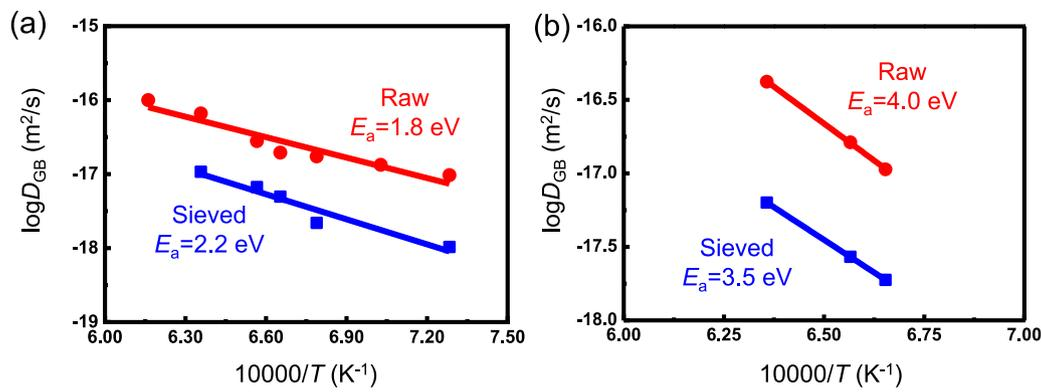
Fig. 4. Arrhenius plot of grain boundary diffusivity  $D_{GB}$  calculated by (a) Johnson's method and (b) Herring's method.
