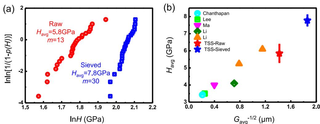
**Fig. 8.** (a) Weibull distribution of measured Vickers hardness for two-step sintered W at  $T_1=1230$  °C for 0 h and then at  $T_2=1180$  °C for 10 h. (b) Comparison of hardness data with the literature reports [4,15,16,41,42].
