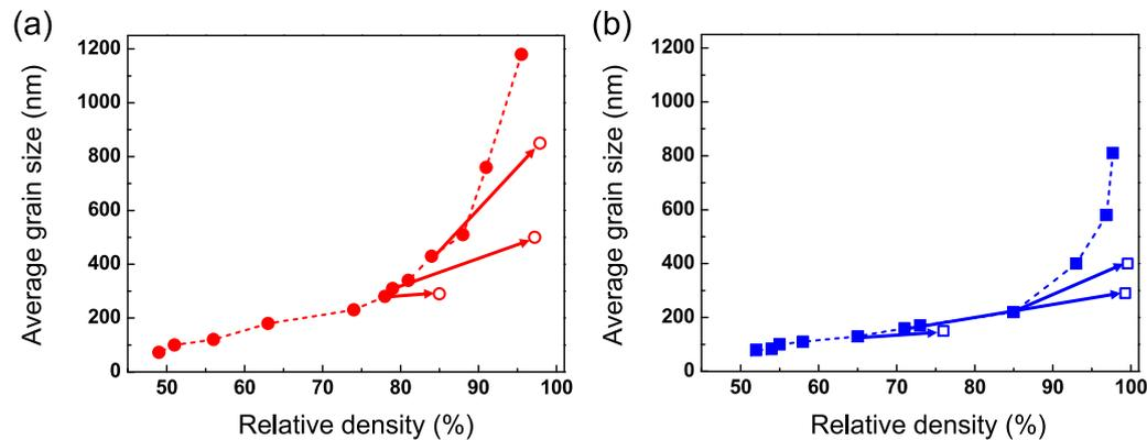
Fig. 5. Grain size-density trajectory of (a) raw-powder and (b) sieved-powder derived samples. Filled symbols denote data from constant-heating-rate sintering without holding and open symbols denote data from two-step sintering. Solid lines with arrows connect the data after the first sintering step to the ones after full two-step sintering schedule. Dash lines are for the guidance of eyes.
