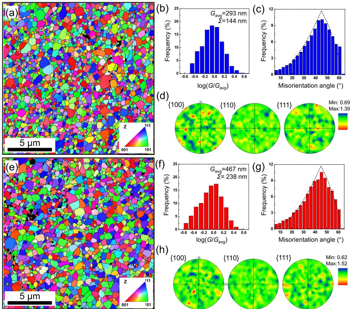
**Fig. 7.** EBSD results of (a-d) sieved-powder, and (e-h) raw-powder derived samples two-step sintered at  $T_1=1230\text{ }^\circ\text{C}$  for 0 h and then at  $T_2=1180\text{ }^\circ\text{C}$  for 10 h. (a, e) Inverse pole figure map, (b, f) normalized grain size distribution, (c, g) distributions of grain boundary misorientation angles (dash lines: Mackenzie's distribution for randomly oriented cubic grains [40]), and (d, h) pole figures.
