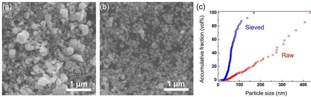
Fig. 1. SEM images of (a) raw and (b) sieved W powders, and (c) their particle size distributions.
