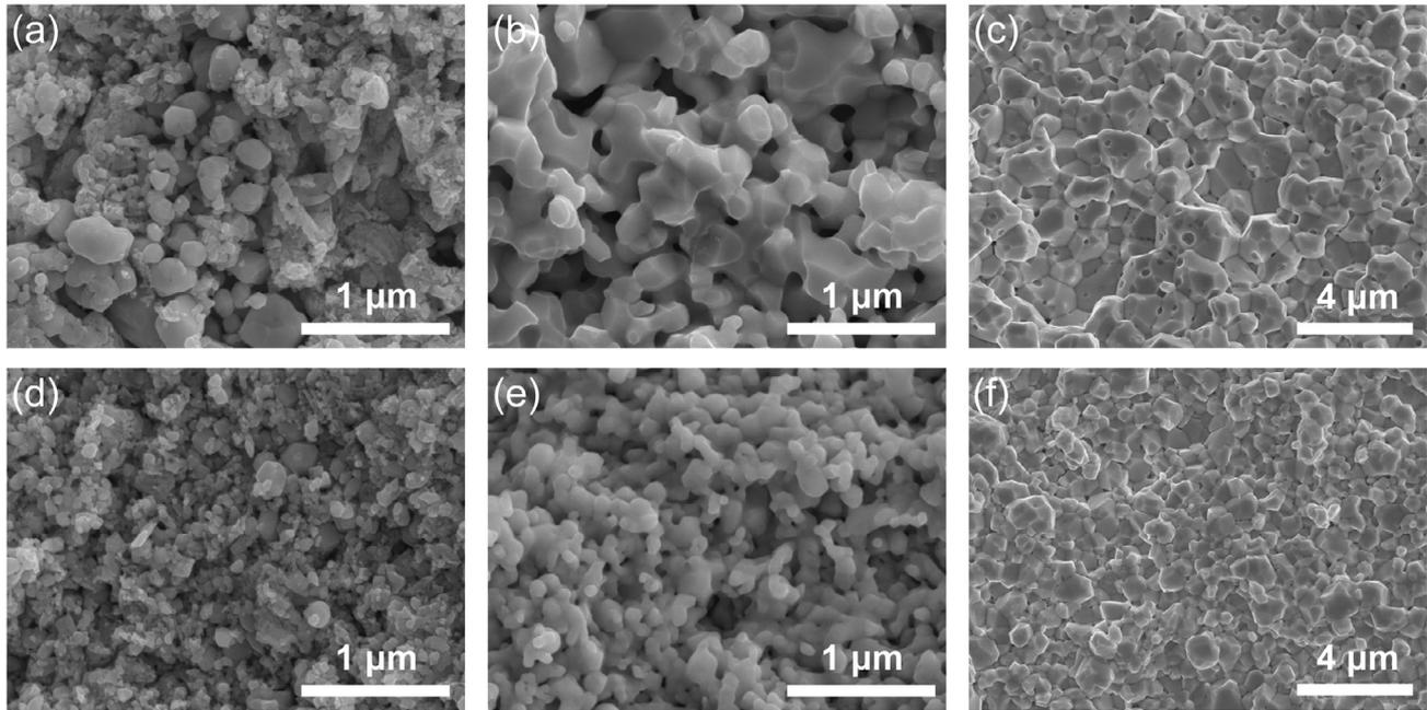
Fig. 2. Microstructures of raw-powder derived samples sintered at (a) 900 °C, (b) 1200 °C, and (c) 1500 °C without holding, and sieved-powder derived samples sintered at (d) 900 °C, (e) 1200 °C, and (f) 1500 °C without holding.
