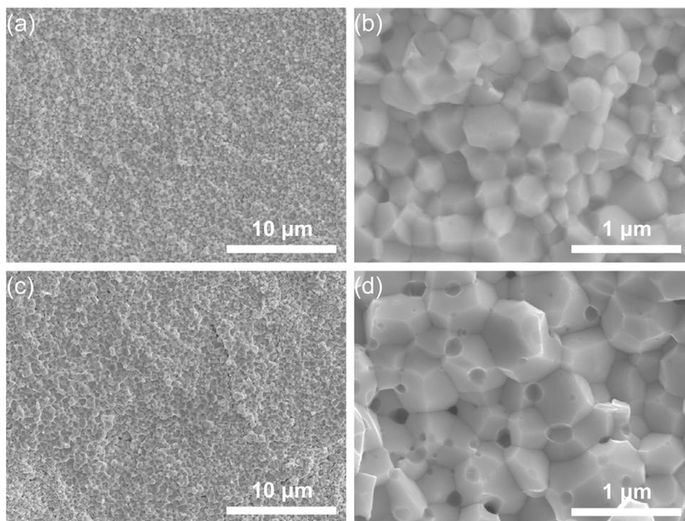
**Fig. 6.** Fracture surfaces of (a, b) sieved-powder, and (c, d) raw-powder derived samples two-step sintered at  $T_1=1230$  °C for 0 h and then at  $T_2=1180$  °C for 10 h.
