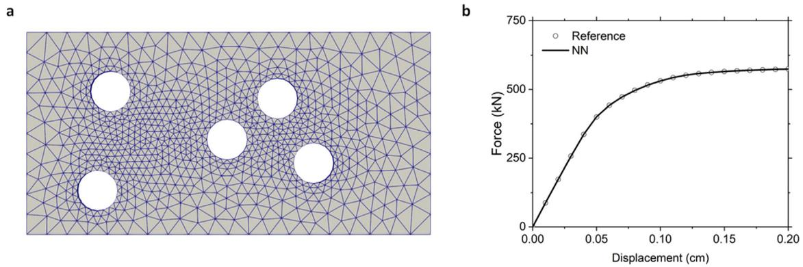
**Fig. 4.** FEM-NN results for a thin-plate geometry that is not included in the training set. (a) FEM mesh in the plate with hole arrangement different from that in Fig. 2(a). (b) Comparison between the reference and FEM-NN-predicted results of sample-level force–displacement response.
