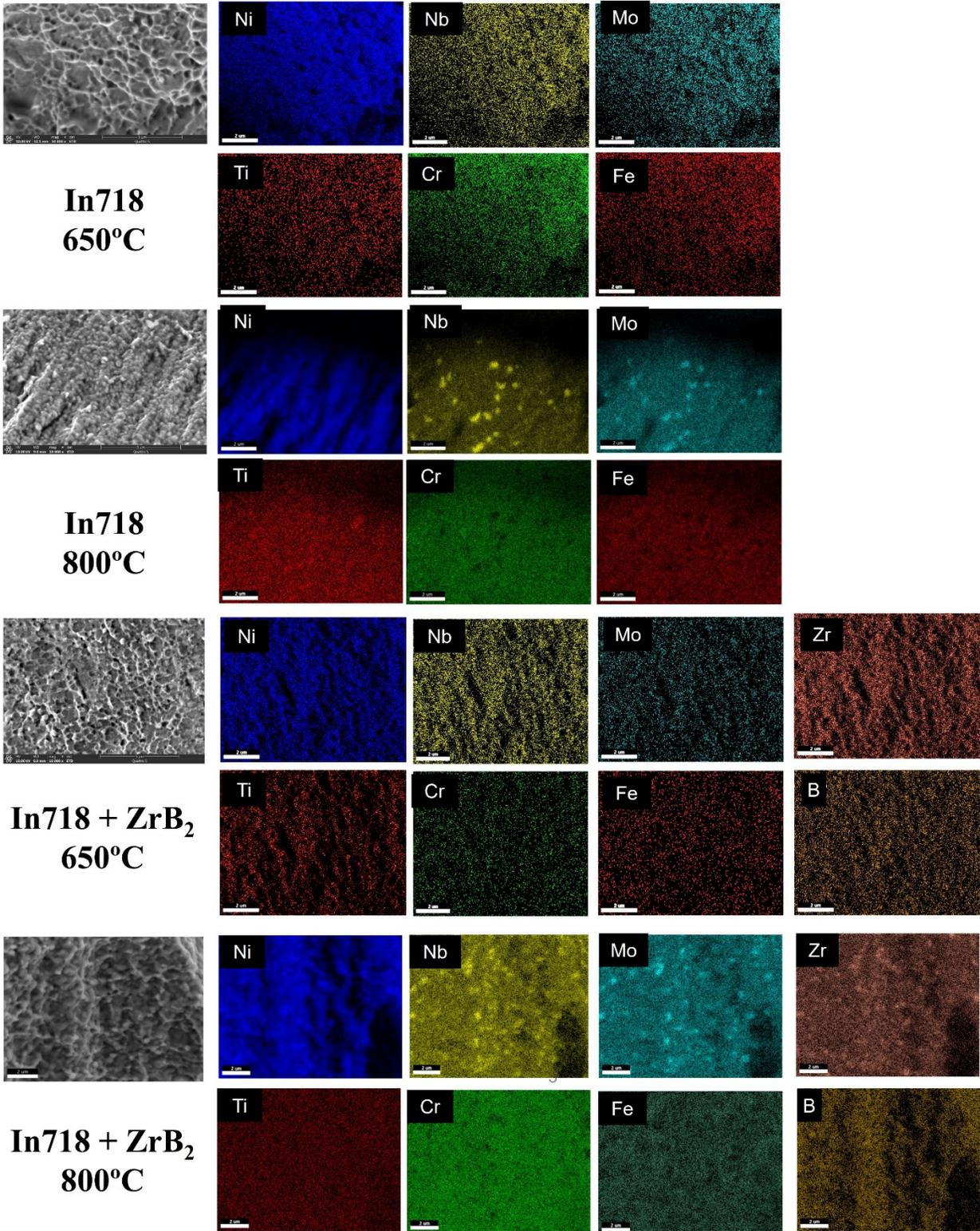
**Fig. S3.** Secondary electron SEM images and EDX mapping analysis obtained from fracture surfaces of samples exposed to tensile testing at elevated temperatures.
