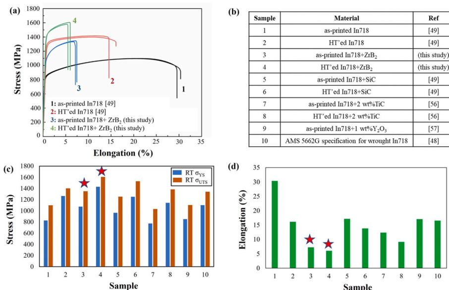
**Fig. 8.** (a) Room temperature tensile stress-strain curves of pure In718 [49] and In718+ZrB<sub>2</sub>, (b) Table listing the sample number vs materials, (c) Comparison of room temperature  $\sigma_{YS}$  and  $\sigma_{UTS}$  of several LPBF'ed In718 and In718-based composites with and without heat treatment, and (d) Comparison of room temperature elongation (%) of several LPBF'ed In718 and In718-based composites with and without heat treatment.
