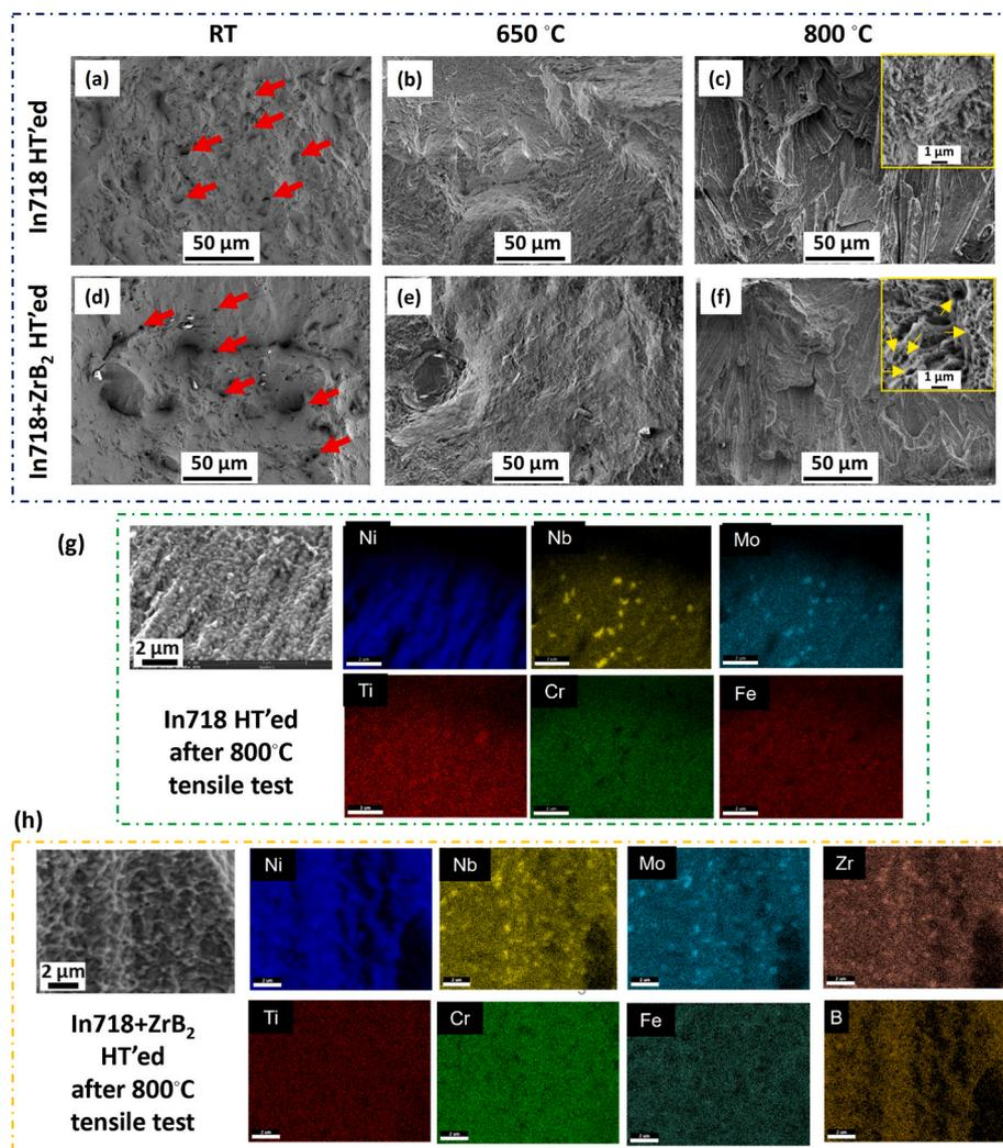
**Fig. 11.** Fracture surface analysis for tensile tests conducted at different temperatures: (a–c) HT'ed In718 and (d–f) HT'ed In718+ZrB<sub>2</sub>, and SEM/EDX mapping analysis obtained from fracture surfaces of (g) HT'ed In718 and (h) In718+ZrB<sub>2</sub> after 800 °C tensile test.
