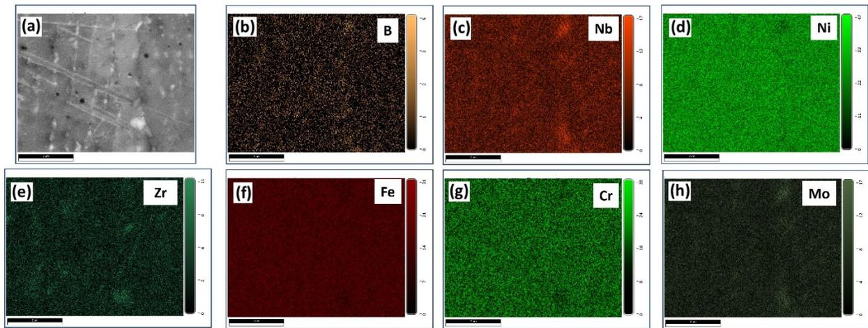
**Fig. S1.** Secondary electron SEM images and EDX mapping analysis obtained from as-printed In718+ZrB<sub>2</sub>.
