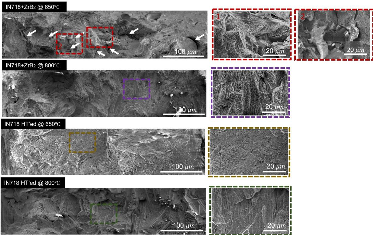
**Fig. S2.** Secondary electron SEM images obtained from fracture surfaces of samples exposed to tensile testing at elevated temperatures.
