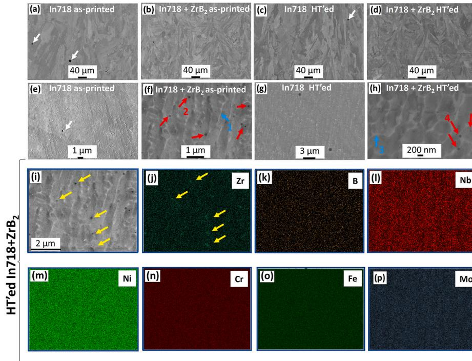
**Fig. 3.** (a–h) Secondary electron SEM images obtained from LPBF'ed samples (white arrows indicate pores, blue arrows indicate Mn–Mo rich regions, red arrows indicate Zr-rich regions), and (i–p) EDX mapping analysis obtained from HT'ed In718+ZrB<sub>2</sub> (yellow arrows indicate Zr-rich regions). (For interpretation of the references to colour in this figure legend, the reader is referred to the Web version of this article.)
