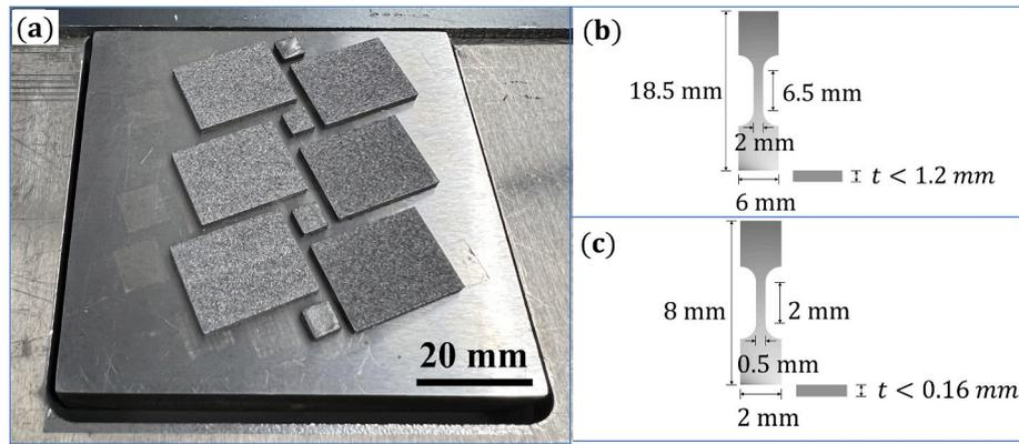
**Fig. 2.** (a) In718+ZrB<sub>2</sub> samples fabricated in EOS M290 SLM printer, (b) Geometry and dimensions of RT tensile specimen machined by wire EDM, and (c) Geometry and dimensions of high-temperature tensile specimen machined by wire EDM.
