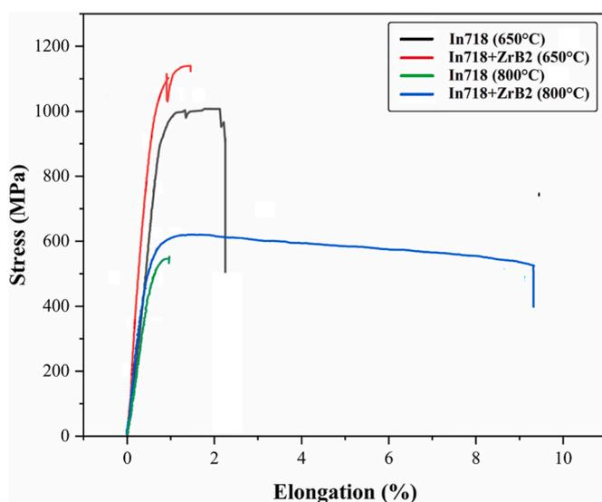
**Fig. 9.** High-temperature tensile stress-strain curves for HT'ed In718 and In718+ZrB<sub>2</sub> samples.
