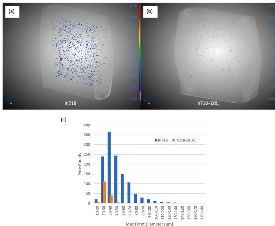
**Fig. 4.** X-ray CT reconstructions displaying pores with diameters >20  $\mu\text{m}$  formed during printing of (a) In718 and (b) In718+ZrB<sub>2</sub> samples. (c) Histogram of pore counts for unfortified and fortified samples organized by maximum Feret diameter.
