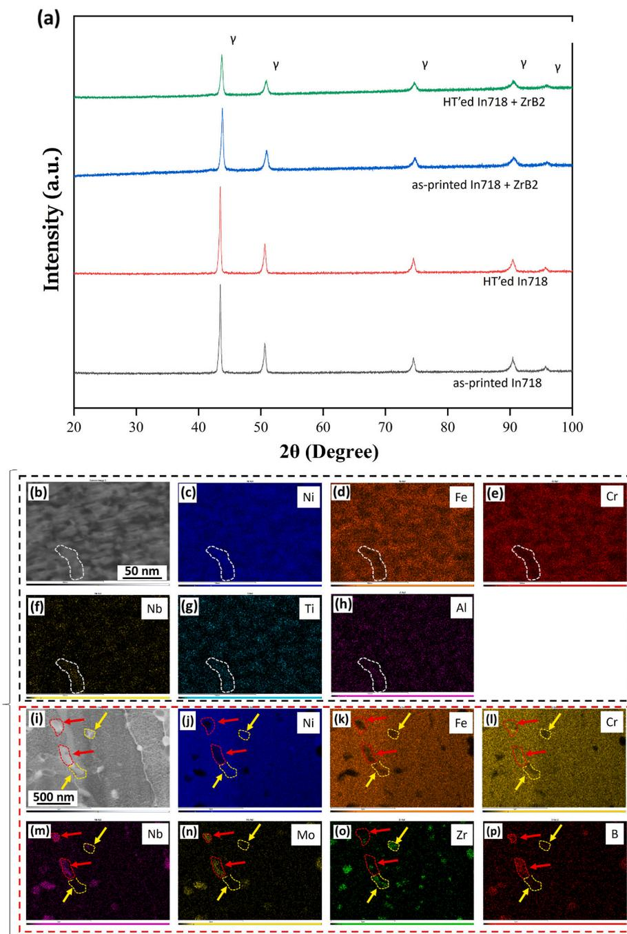
**Fig. 5.** STEM/EDX mapping analysis obtained from HT'ed In718+ZrB<sub>2</sub> showing: (a–g)  $\gamma'$  and  $\gamma''$  precipitates (white dashed regions) and (h–o) (Nb, Mo, Cr)-based borides and (Zr, Ni)-based intermetallic nanoparticles (red arrows indicate Nb, Mo, Cr, B-rich regions, yellow arrows indicate Zr, Ni-rich regions). (For interpretation of the references to colour in this figure legend, the reader is referred to the Web version of this article.)
