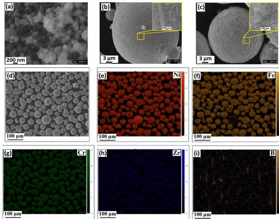
Fig. 1. SEM micrographs of (a) commercial  $ZrB_2$  powders, (b) In718 particle surface before blending, and (c)  $ZrB_2$  decorated In718 particle surface after blending. (d–i) SEM micrographs and EDX mappings of In718+ $ZrB_2$  powders after blending.
