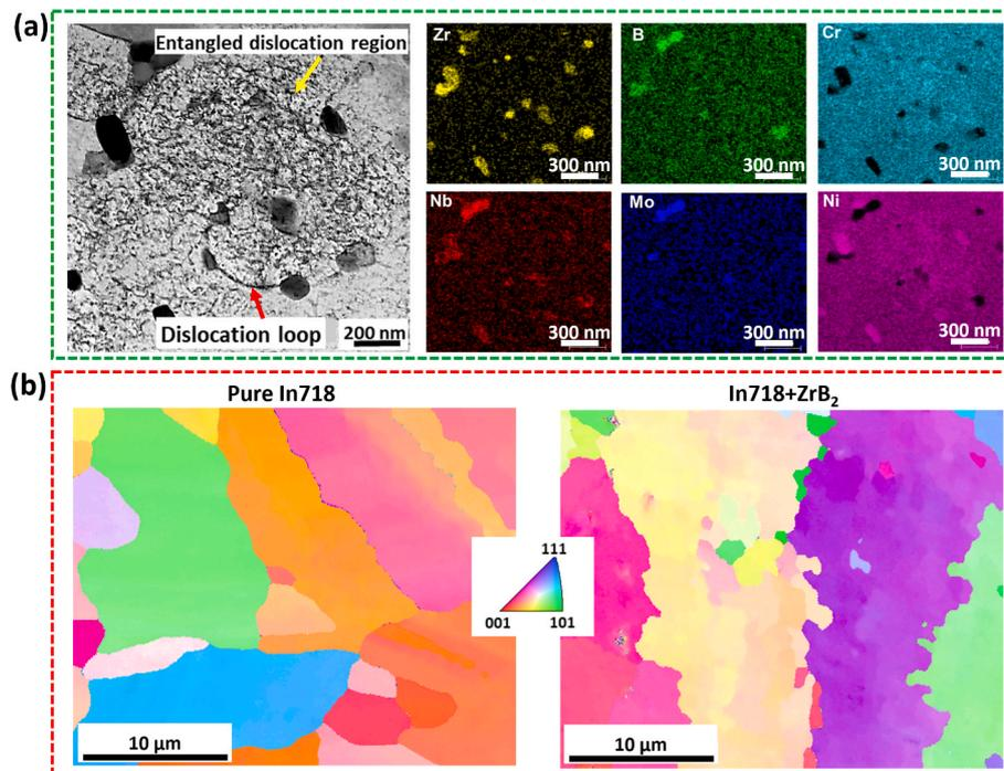
Fig. 10. (a) STEM image and EDX mapping obtained from HT’ed In718+ZrB<sub>2</sub> after 800 °C tensile test showing dislocation loop and entanglement in the microstructure and (b) EBSD maps obtained from HT’ed In718 and In718+ZrB<sub>2</sub> showing the difference of grain boundary morphologies.
