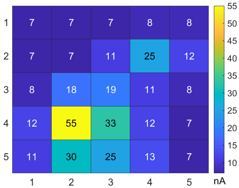
Supplementary Fig. 46 | Raw data for current distribution of humidity sensor array. Original current distribution of 5×5 humid sensor array in none-contact finger localization experiments.
