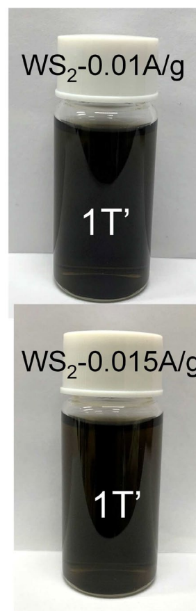
Supplementary Fig. 4 | Characterization of exfoliated WS 2 . Raman spectra of WS 2 exfoliated under discharge current densities of 0.01 A g -1 and 0.015 A g -1 , right-side show the corresponding photographs of exfoliated solution.
