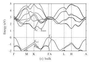
FIG. 1. Band structures of monolayer (a), bilayer (b), and bulk (c)  $MoS_2$  from QSGW calculations.
