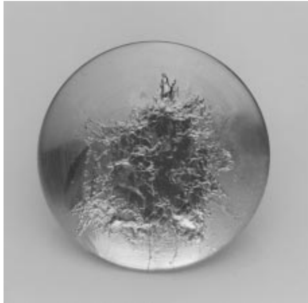
Figure 52. Frascati Tokamak limiter of a tungsten coated TZM mushroom type (60 mm in diameter) after plasma transient events. (Figure provided by G. Maddaluno, ENEA, Frascati.)
