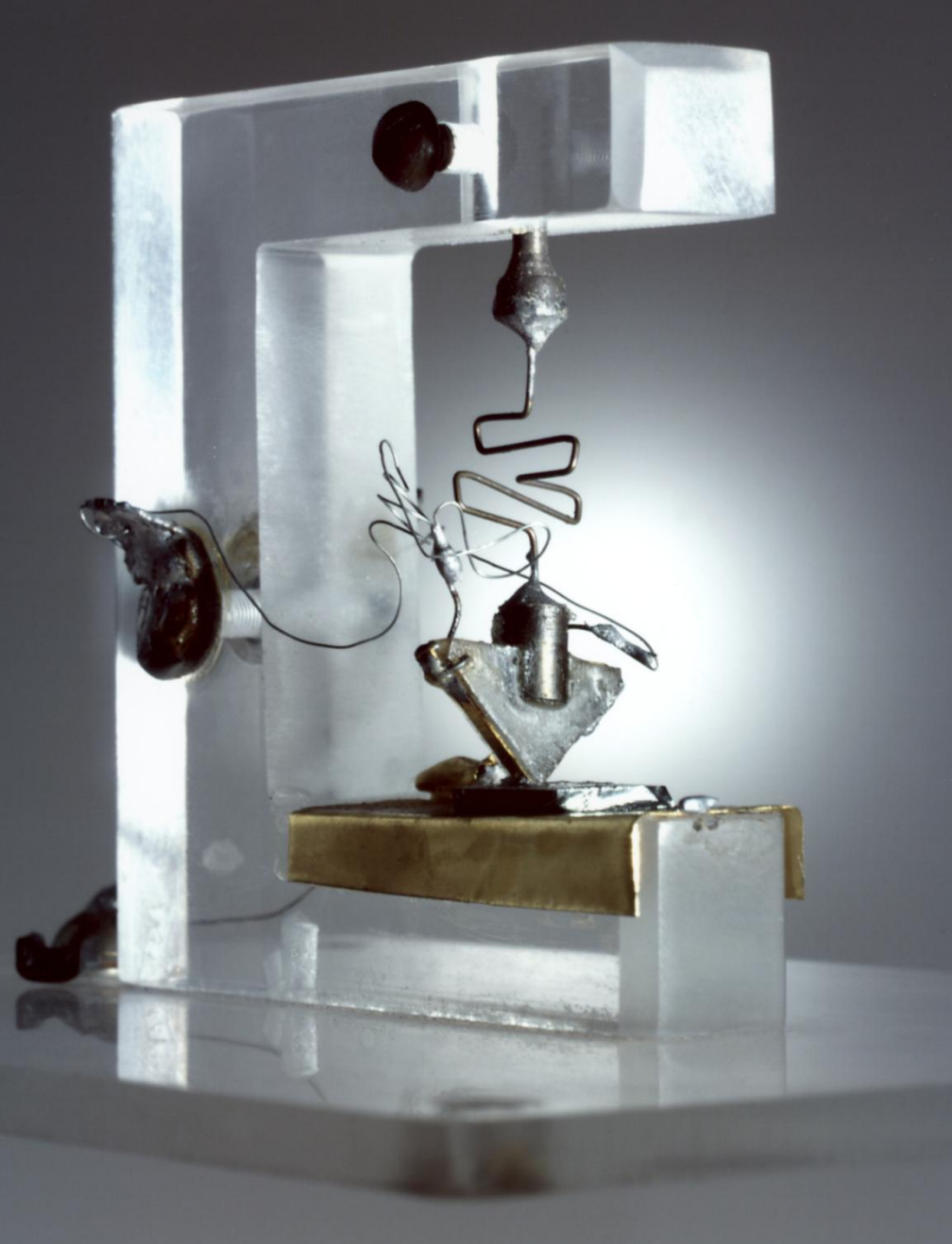
First semiconductor transistor (1947, Bell Labs)
