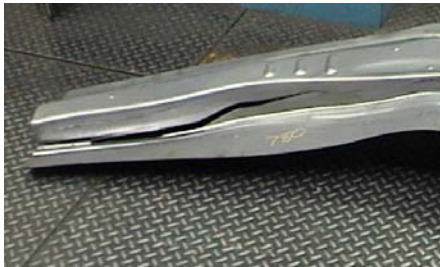
Failure under Stretch-bending (DP780 steel Shown)
