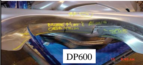
Formed Part Showing Edge Cracking
