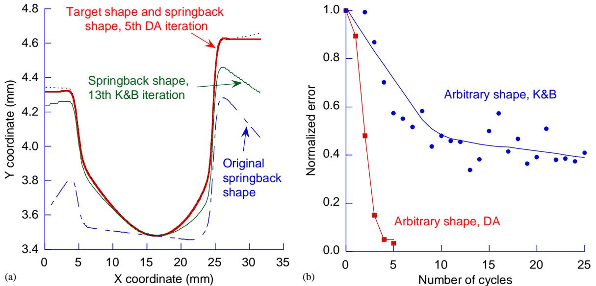
Fig. 7. Arbitrary 2D shape results: (a) Part shapes, DA method; (b) convergence behavior of DA and K&B compared.
