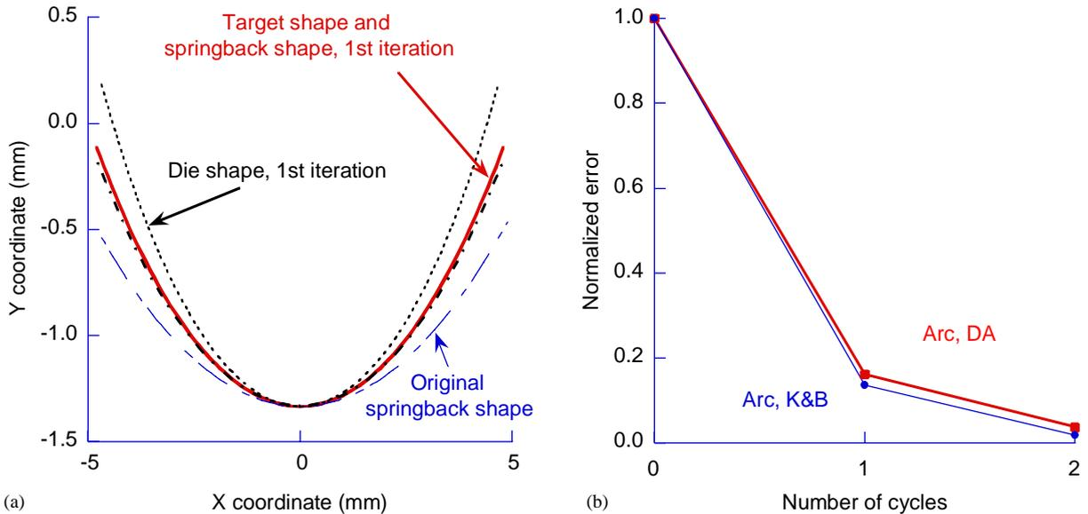
Fig. 4. Arc-bending results: (a) Die and part shapes, DA method; (b) convergence behavior of DA and K&B compared.
