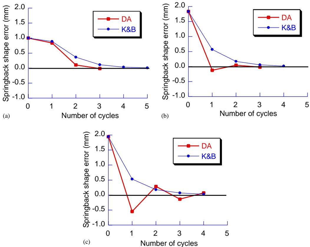
Fig. 11. Dependence of K&B and DA on deformation geometry. The target shape is the shape with  $\Delta y$  equal to (a) 1 mm, (b) 2 mm, (c) 2.5 mm.
