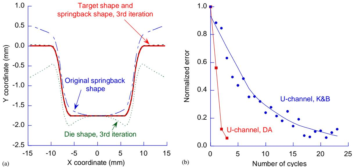
Fig. 5. U-channel bending results: (a) Die and part shapes, DA method; (b) convergence behavior of DA and K&B compared.
