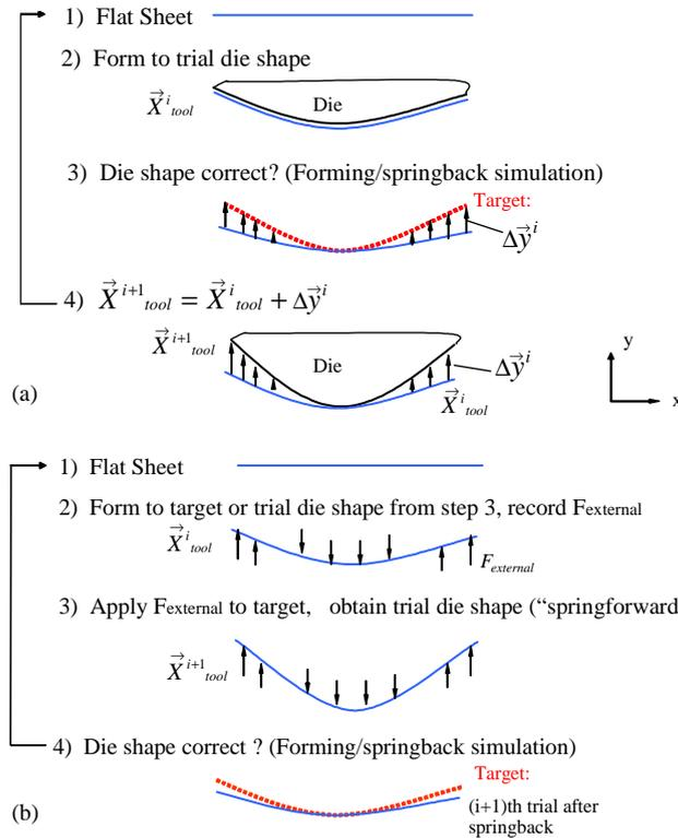
Fig. 1. (a) Flowchart of DA method; (b) flowchart of K&B method.
