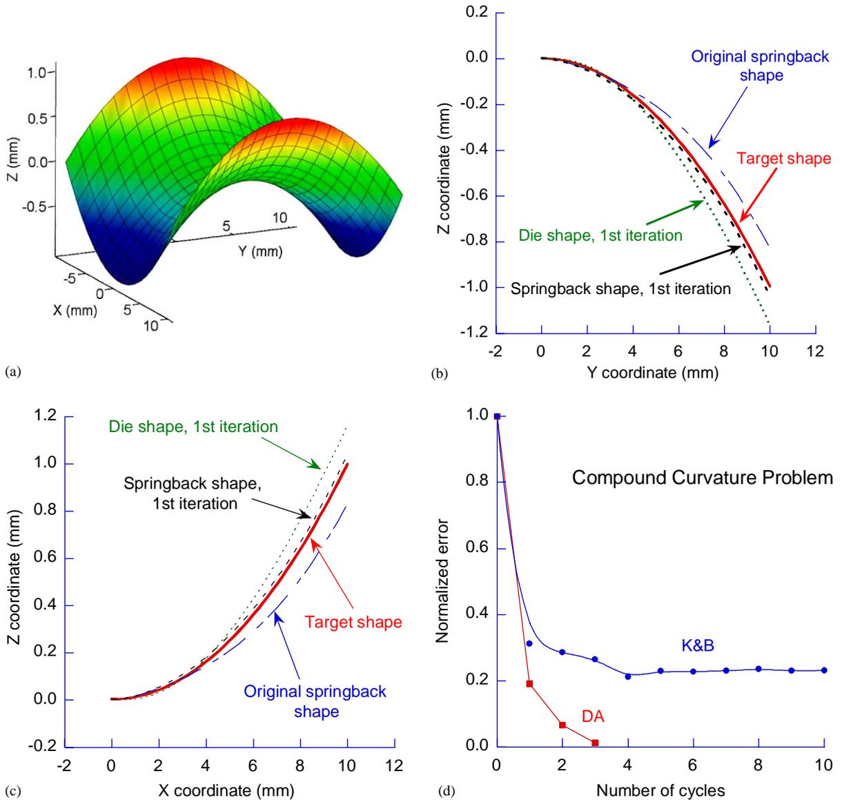
Fig. 6. Three-dimensional compound curvature bending results: (a) Target part shape; (b) die and part profiles along the Y–Z symmetry plane, DA method; (c) die and part profiles along the X–Z symmetry plane, DA method; (d) convergence behavior of DA and K&B compared.
