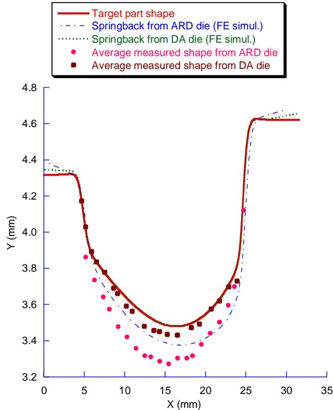
Fig. 8. Experimental validation of the DA method.
