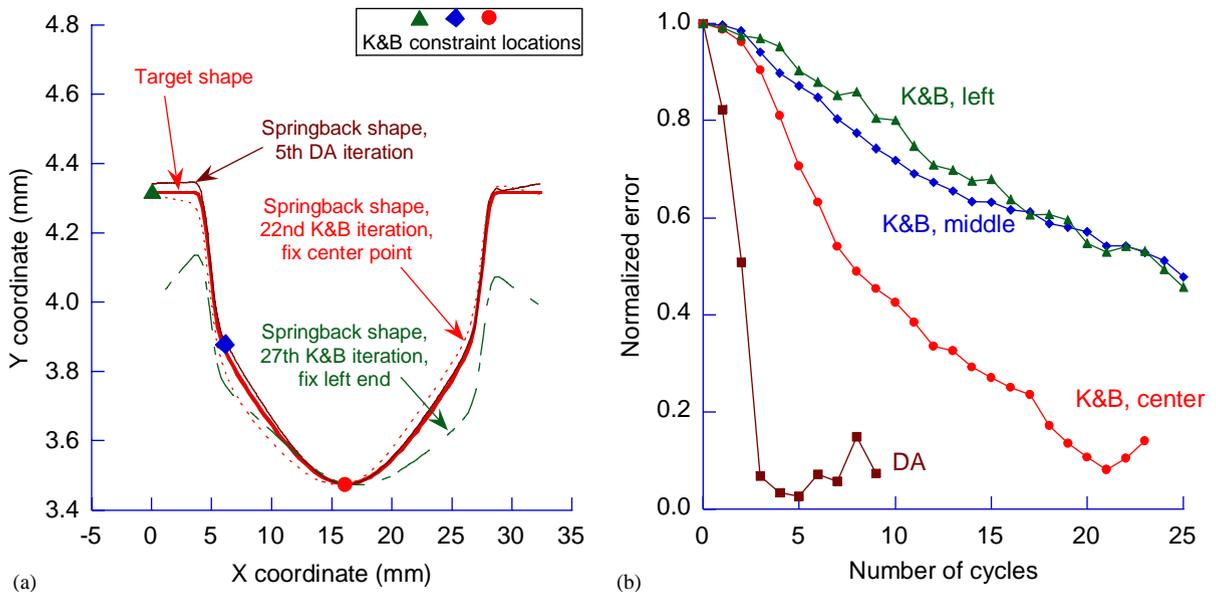
Fig. 9. Symmetric arbitrary 2D shape results: (a) Part shapes; (b) convergence behavior of DA and K&B compared.
