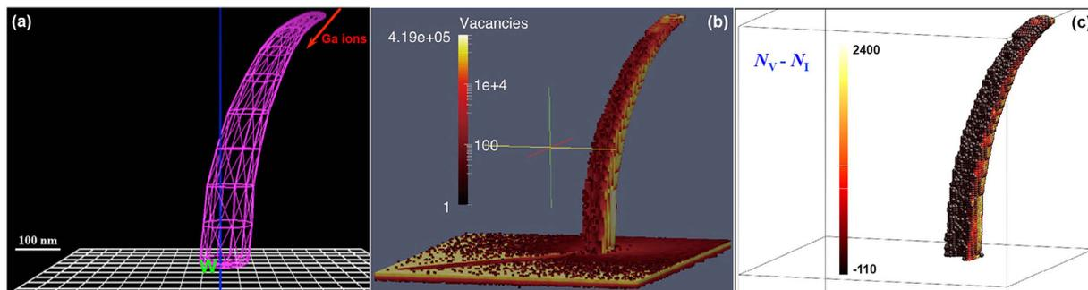
**Figure 9.** The (a) 3D surface mesh with FETM geometric method, (b) vacancy spatial distribution and (c) remaining excess vacancies for a bent W nanowire under randomly distributed Ga ion sputtering with an incident direction of 40 degrees and an energy of 150 keV.
